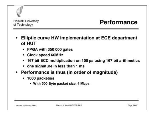
An example of the speed of digital signatures made in HW is one of our projects at HUT. In GO-SEC –project, we have implemented elliptic curve on FPGA size and speed listed above. With 167 bit keys, the HW is capable of performing about one multiplication in 100 us. This leads roughly about 1 ms time per digital signatures.
